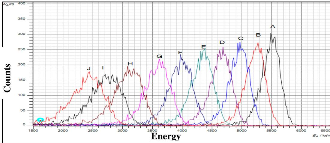
**Figure 6.** Measured Loss Energy of Alpha Particles in Gold Absorber Using Am-241 Source
