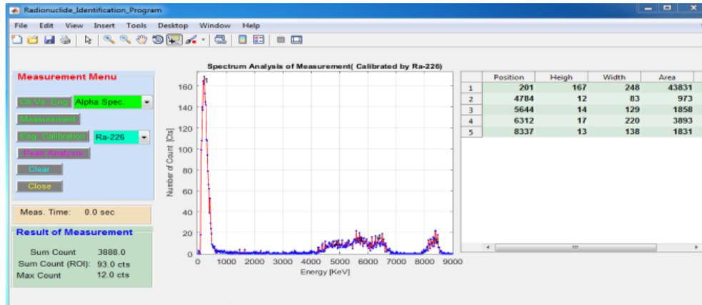
Figure 4. The Result Interface of in Peak Analysis Radionuclide Identification Program
