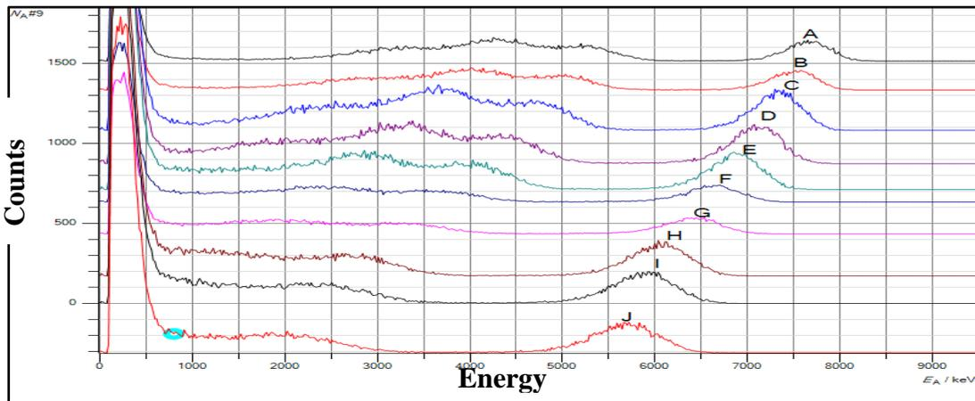
Figure 9. Energy loss of Alpha Particles in Gold Absorber Using Ra-226 Source
