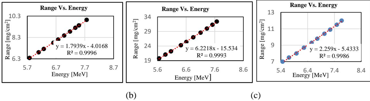
**Figure 11.** Range and Energy Relation of Alpha Particle (a) in Air Medium (b) in Gold and (c) in Aluminium using Ra-226 Source
