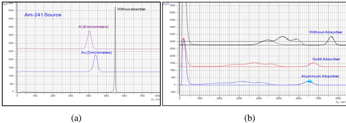
**Figure 12.** Energy Loss Spectra of Alpha Particles at 100 mbar using (a) Am-241 and (b) Ra-226 Source
