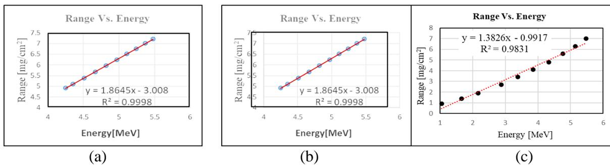
**Figure 8.** Range and Energy Relation of Alpha Particle (a) in Air Medium (b) in Gold and (c) in Aluminium using Am-241 Source
